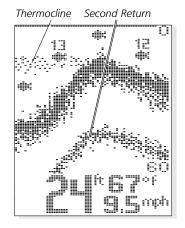
usually appears as a dense cluster of individual dots. If the return meets certain additional criteria, a fish symbol is assigned. There are three different size fish symbols used to indicate the intensity of the sonar return. While signal intensity is a good indicator of relative fish size,
